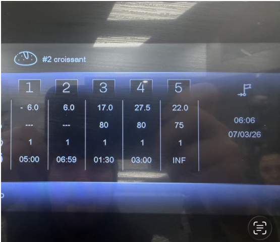
Everlasting retarder/proofer programme shown; humidity subsequently standardised to 75%.
